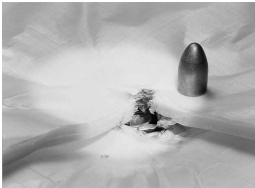
Figure 13 Stopped 9 mm Parabellum bullet in a soft ballistic package.
