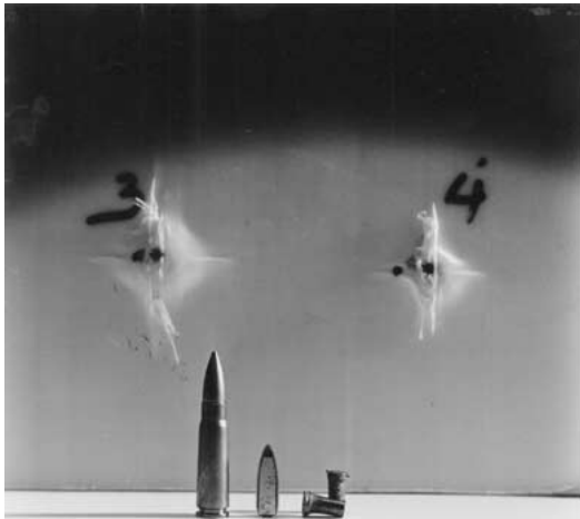
Figure 14 Panel tested against 7.62 \times 38 Mild Steel Kalashnikov AK47.
